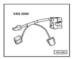
Special tools, workshop equipment, test equipment and auxiliary items required Airbag adapter VAS 5094
