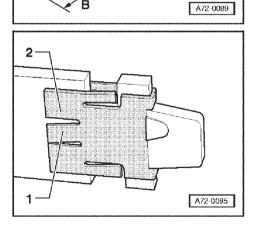
→ The spring -1- of the retaining clip -2- must face the seat.
