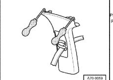
— To facilitate disassembly use two assembly hooks -2-.
