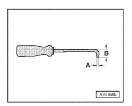
Bend a flat screw driver with dimensions A approx. 3 mm and B approx. 10 mm.
