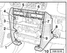
– Unclip the switch panel trim, starting at the bottom edge arrows-.
