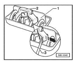
Use screwdriver -3- to lever out bracket -2- from glove compartment actuation -1- on left and right side in direction of arrow.
