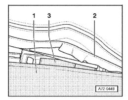
When installing the seat extension cover -1-, the fabric -2- must be pushed back and engaged in the seat shell with tab -3-.
