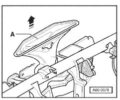
Removing outer right attachment point
