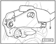
Remove mounting plate -1- on opposite side and pull out transfer shaft -2-.
