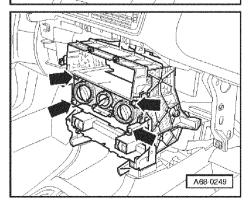
Unscrew bolts -arrows- for heater controls.
