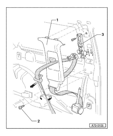
Height adjuster must engage audibly in each of the 5 possible positions (including top position).
