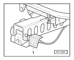
Grip underside of Bowden cable cover -1- and pull downwards and forwards.
