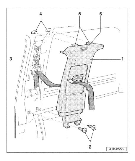
♦ After installing trim ensure seal is seated correctly.
