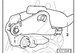
Remove mounting plate -1- on opposite side and pull out transfer shaft -2-.
