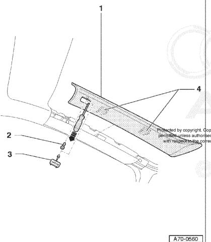
Use screwdriver -5- (improvised tool = > Fig. 1) to grip A-pillar trim -1- in cut-out and unclip trim at upper clamp in direction of arrow.
