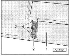
Push the fabric cover with plastic channel -2- into the padding 1-.
