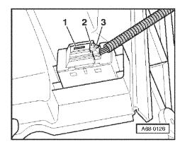
Fig.1 Detaching connector for passenger airbag key switch.
